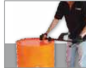
Removable handle used as a drum wrench
