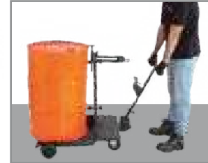
Removable handle used for moving the trolley
